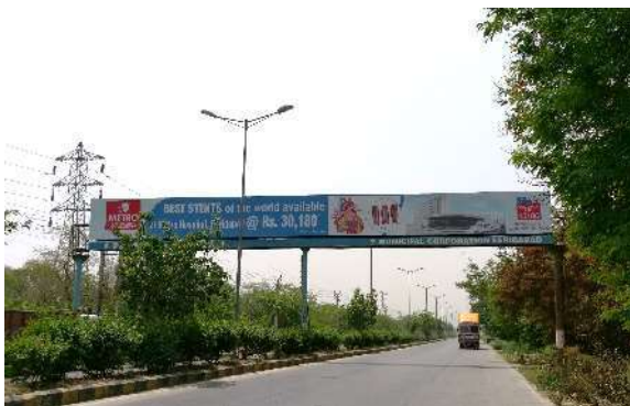
Exhibit 4-31: An overhead hoarding causing distraction to driver
